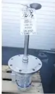
TURBO-MIXER Agitator with Turbo-Mixer Type DFHD 4/10 and motor 1,5 KW
