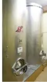
8.200 liter liter storage tank, wine tank round with flat bottom with 3% sloping
