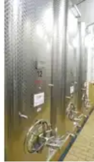
10.230 Litres DEFRANCESCHI Storage Tank/Wine tank cubical with flat bottom and 3 % incline
