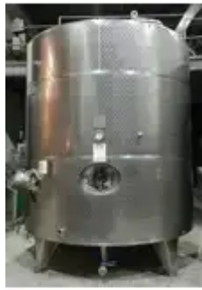
Milk Tank 12.000 Liter in AISI 3041 with agitator
