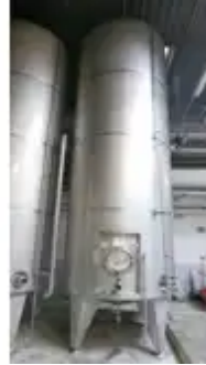
25.000 Liter Storage Tank with insulation, vertical in V2A
