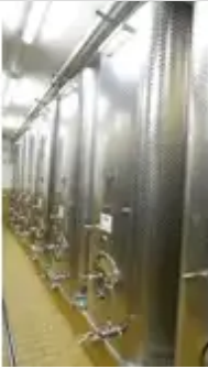
DEFRANCESCHI 6.960 Litres cubical Storage tank/wine tank with flat bottom and 3 % incline
