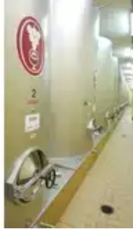
13.600 liter liter storage tank, wine tank round with flat bottom with 3% sloping
