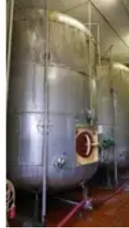
23 000 liter Sparkling Pressure Tank / Sparkling Cooling Tank 8 bar
