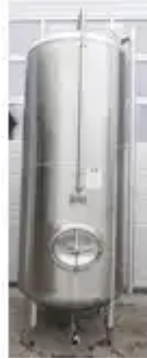
3.207 Liter Storage Tank/ Pressure Tank/ Beer Tank to 2 Bar
