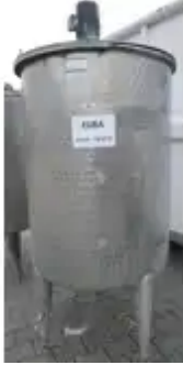
800 Litres Storage Tank with Agitator Mixer
